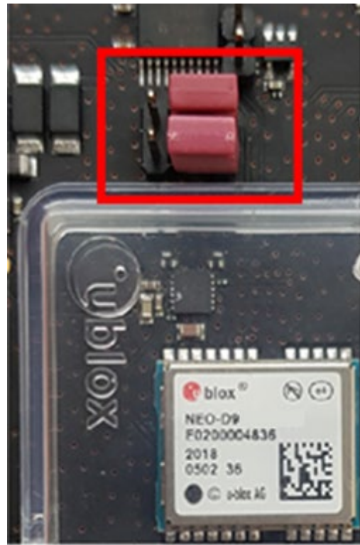
The ZED-F9P receives the correction data on UART2.
