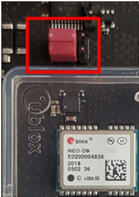
The ZED-F9P receives the correction data on UART1.
