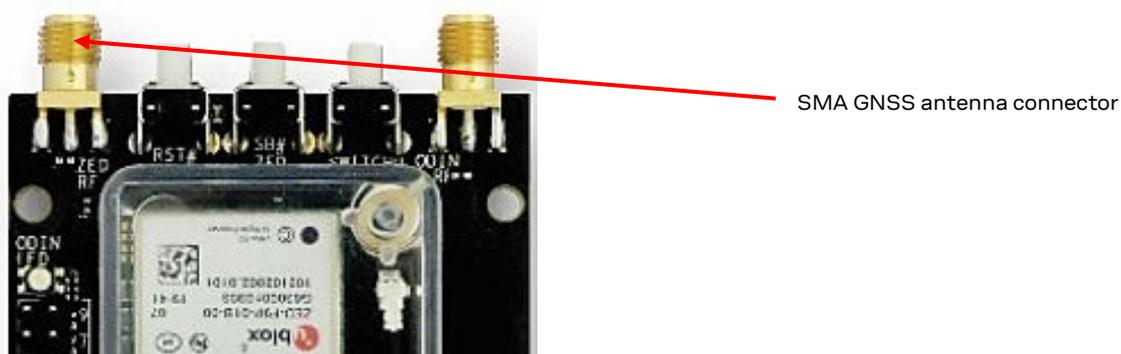
Figure 12: GNSS antenna connector
