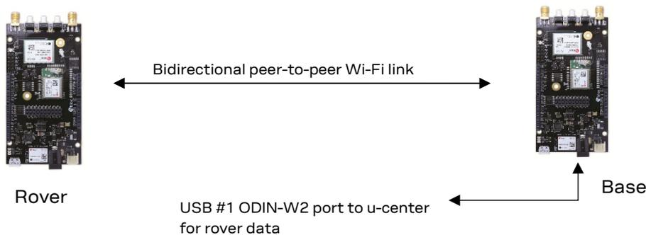
**Figure 26: Reference and rover C099-F9P set up**
