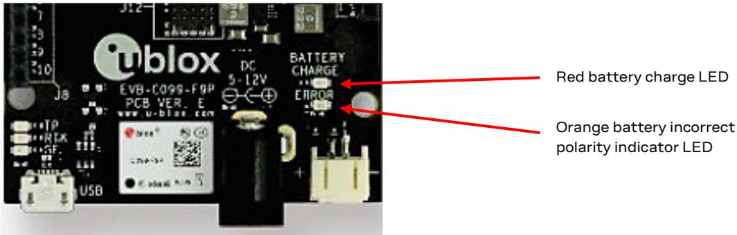
Figure 11: Battery charge status LED
