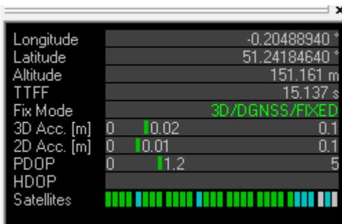
Figure 39: u-center Data view RTK FIXED indication
