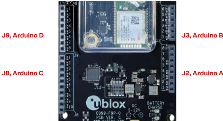
Figure 54: C099-F9P Arduino connectors
