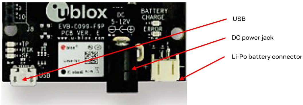
Figure 9: Power connections
