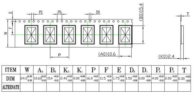
Figure 20 – BMD-340-A-R-00 and BMD-340-A-R-01 carrier tape dimensions
