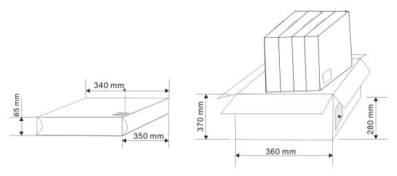
Figure 19 - Reel cartons used for type number BMD-340-A-R-00 and BMD-340-A-R-01
