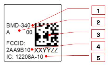
Figure 13: Module marking for type number BMD-340-A-R-00
