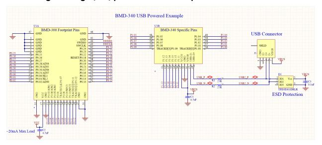
Figure 9: USB-powered HV mode example
