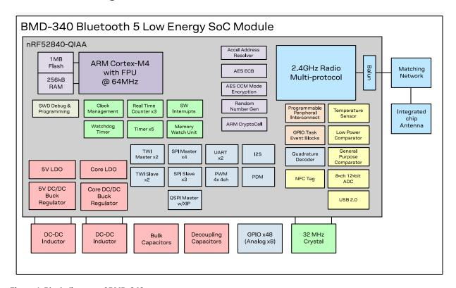
Figure 1: Block diagram of BMD-340
