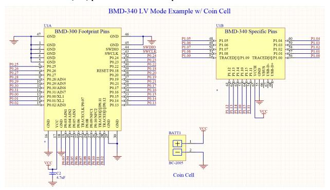
Figure 7: LV Mode w/ Coin Cell Example
