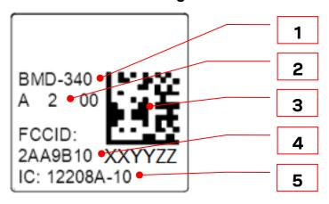
Figure 14: Module marking for type number BMD-340-A-R-01
