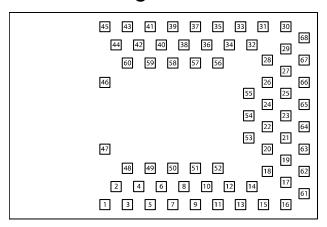
Figure 2: BMD-340 Pin assignment (Top view)
