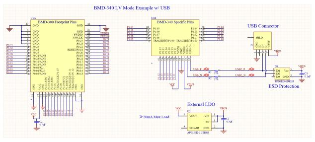
Figure 8: LV Mode w/ USB and external regulator
