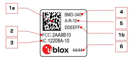
Figure 15: Module marking for type number BMD-340-A-R-10
