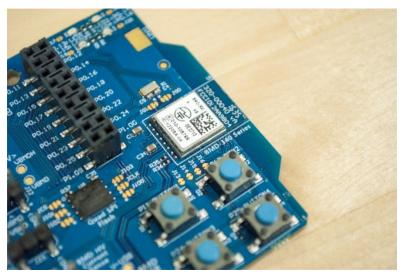
Figure 4: BMD-300 module soldered to BMD-340 footprint
