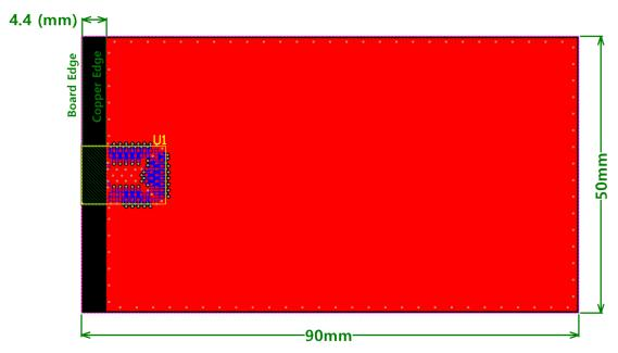
Figure 16: BMD-340 RF example based on the evaluation board
