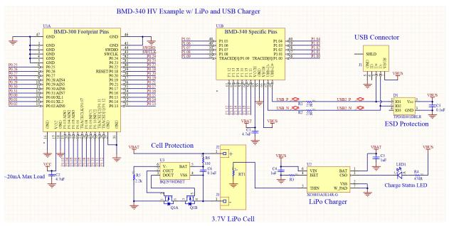
Figure 10: LiPo-powered HV example with USB charger
