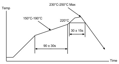
Figure 23: Reflow Profile for Lead Free Solder
