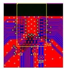
Figure 6: BMD-340 two-layer fan-out example
