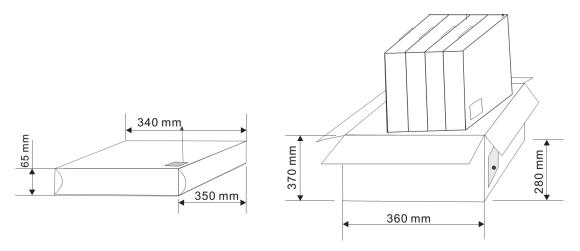
Figure 13: Reel cartons used for type number BMD-300-A-R-00
