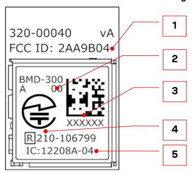
Figure 5: Module marking for type number BMD-300-A-R-00
