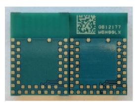
Figure 7: Bottom data matrix and marking example on type number BMD-300-A-R-20
