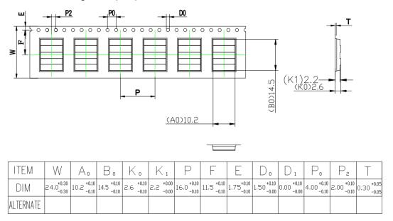
Figure 14: BMD-300-A-R-00 carrier tape dimensions
