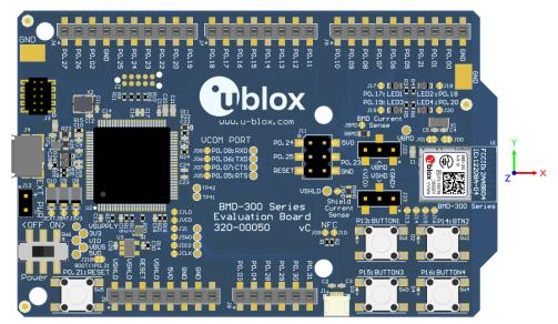
Figure 9: BMD-300 evaluation kit X-Y-Z orientation
