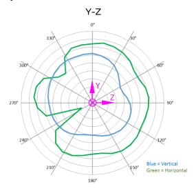
Figure 12: Y-Z plane antenna pattern
