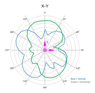
Figure 10: X-Y plane antenna pattern
