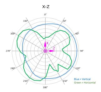
Figure 11: X-Z plane antenna pattern
