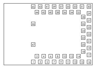
Figure 2: BMD-300 pin assignment (top view)
