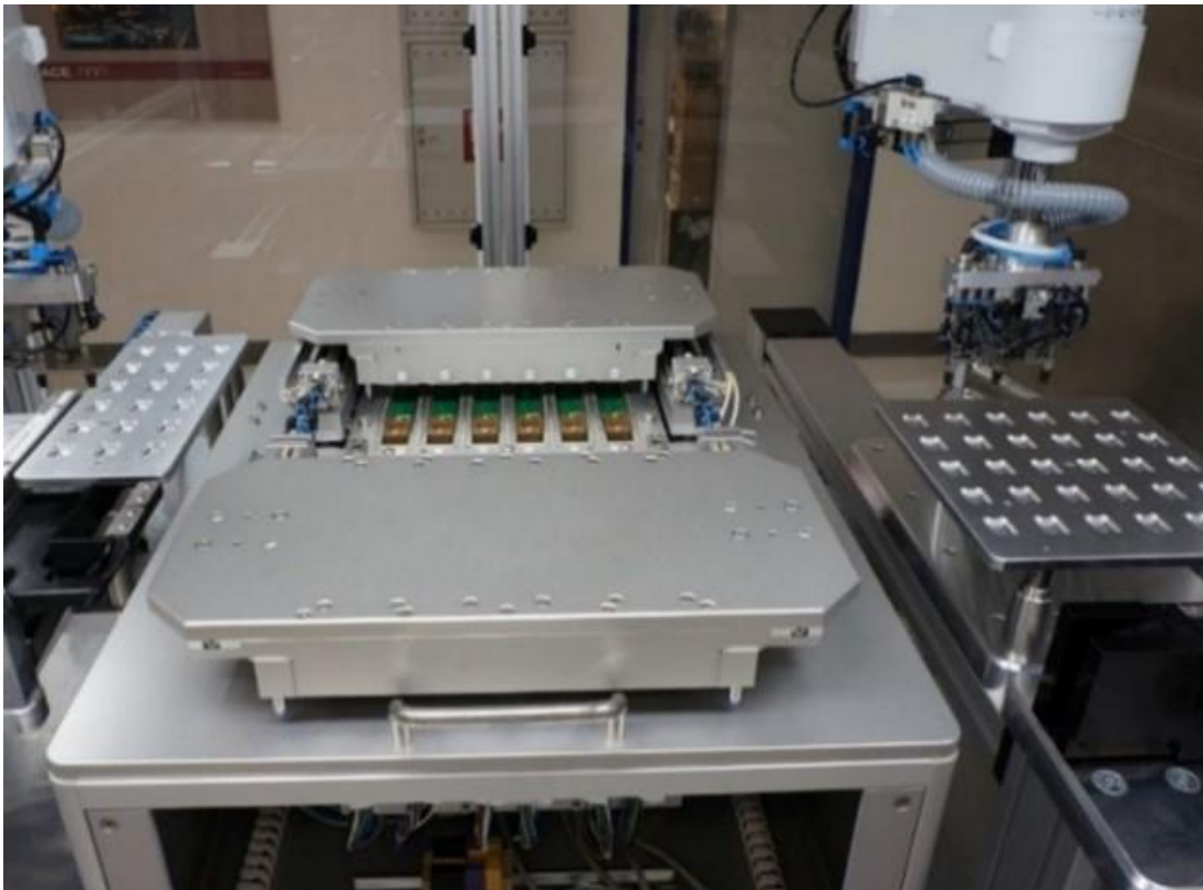
Figure 32: Automatic test equipment for module test
