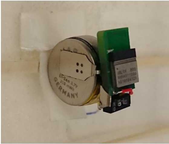
Figure 38: A tiny ANNA-B1 application including coin cell battery with the range of about 100 m, size 7.5 x 12 mm
